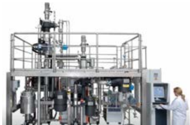
Wiped Film and Short Path Evaporator with control system/visualisation
